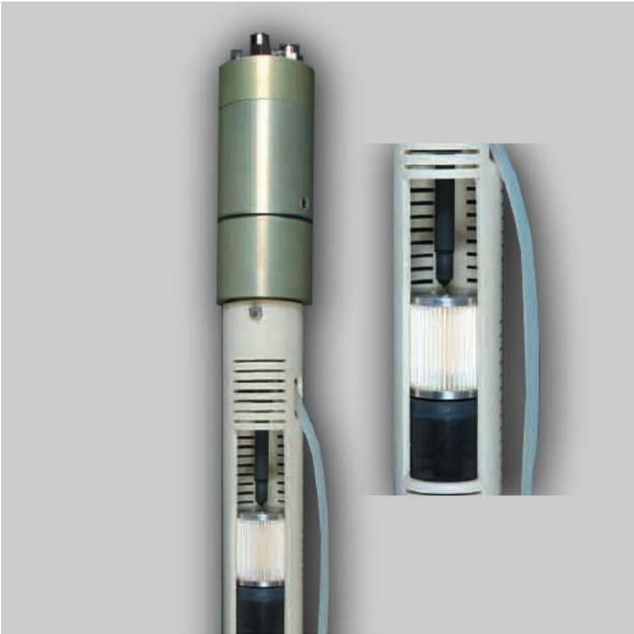
*All-in-one pump and skimmer assembly for 2" and 4" wells.*
