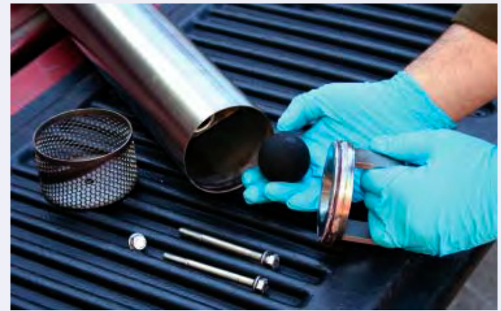
Bottom-loading pump, TR-975, disassembled.
